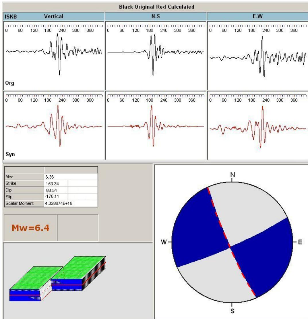
Figure 3. Focal mechanism solution of the mainshock.
